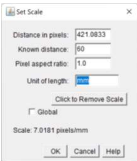
Figure 11. Set Scale options. Since the distance of of the drawn line is known to be 60 mm it is adjusted accordingly.
