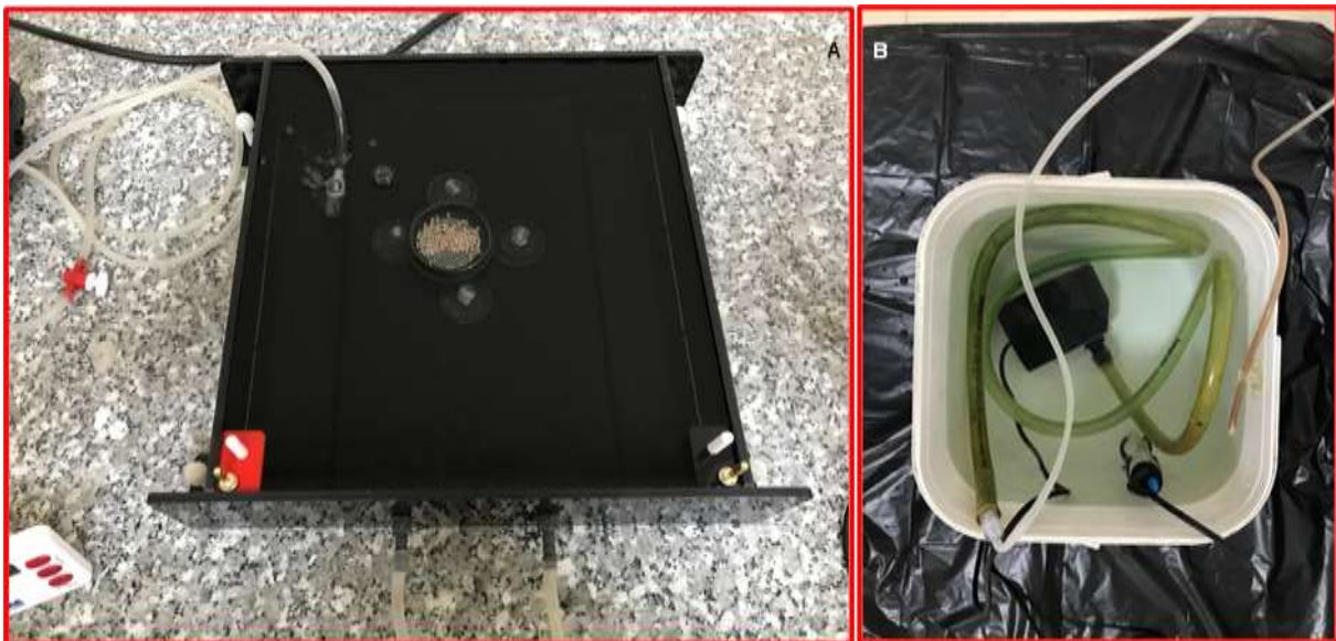
Figure 6. Placing egg tumbler to the electrophoresis tank (A) with aeration supply and recirculation system (B) to keep the tank temperature stable
