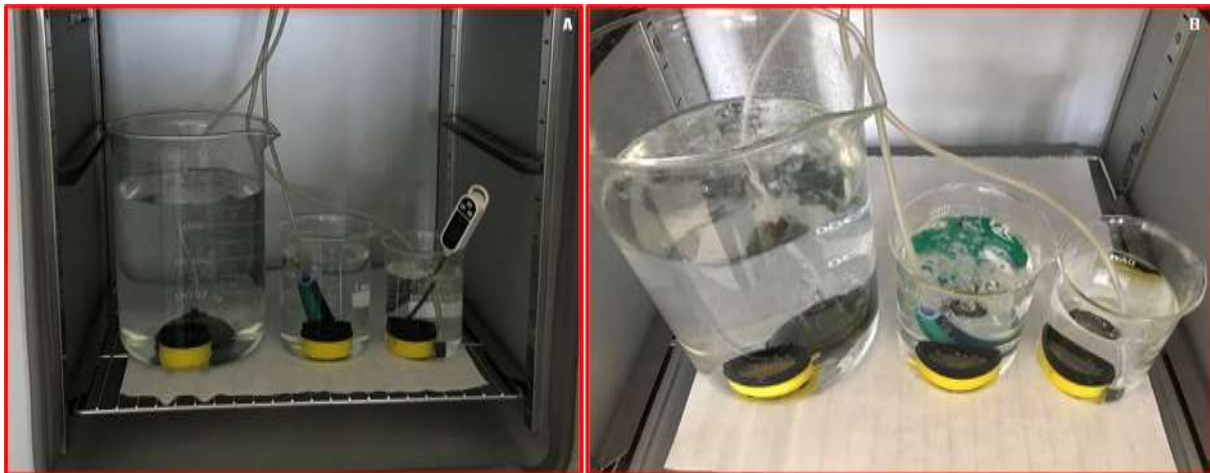
Figure 8. Placing egg tumbler to different sizes of beakers in the oven (A) and aeration supply in the beakers (B).
