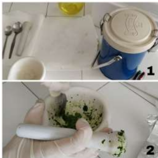
Figure 2. Grinding initial samples 1) Nitrogen container and other equipment required for grinding the initial samples 2) Grinding the tomato leaf with liquid nitrogen by using a mortar and pestle
