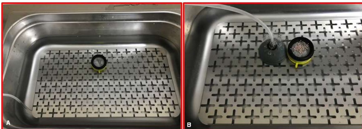
Figure 4. Direct (A) and airstone (B) aeration supplies in experimental system for the heat shock method
