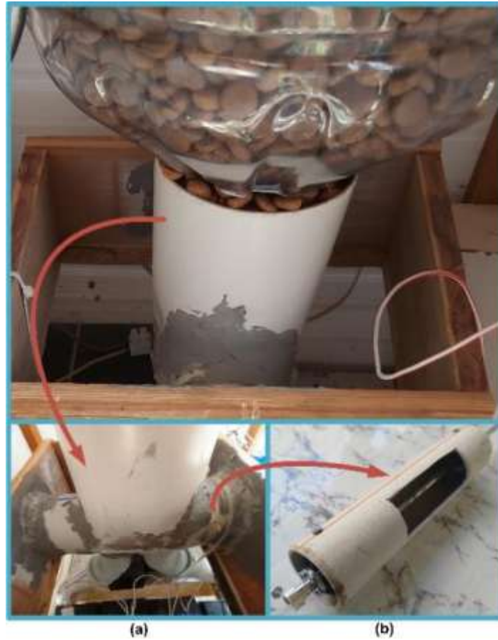
Figure 8. (a) Photograph of two-way splitter, (b) Photograph of food portion dispenser Proposed system's electrical connection and control unit are shown in Figure 9.
