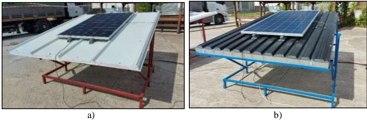
Figure 4. a) PV and b) PV/T systems
