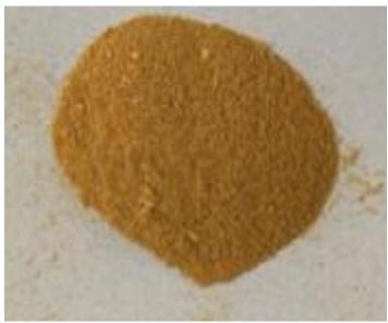
Figure 3. Film sample pulverized by cryogenic crusher
