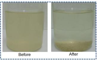
Figure 5. Flocculation process at laboratory
