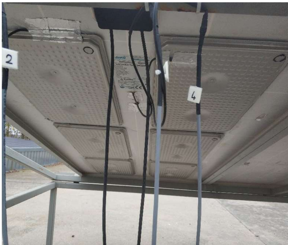
Figure 3. Modules Using Phase Change Material
