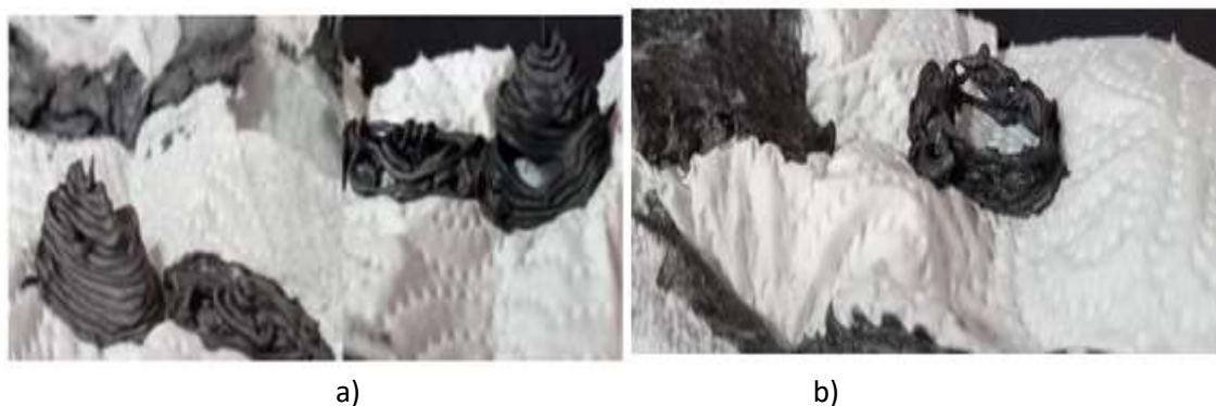
Figure 3. a) Three-dimensional printer output of 11.7% graphite powder reinforced bioplastic b) Printout of 10% fine sand and 15% graphite powder reinforced bioplastic.
