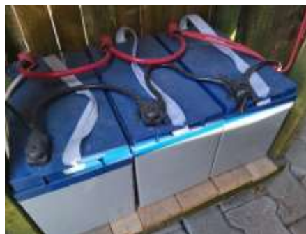
Figure 9. The battery group of the solar-based automatic pet feeder and water dispenser in use
