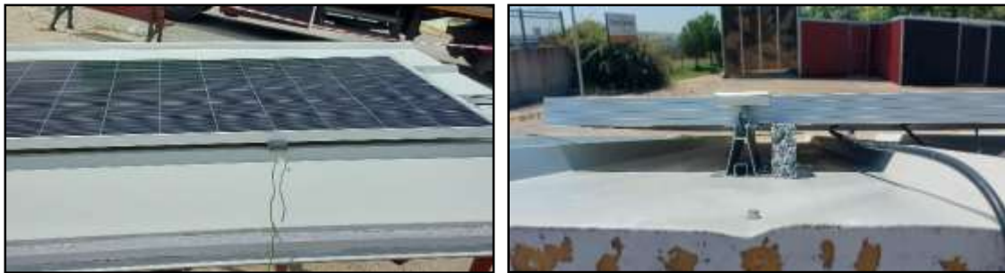
Figure 9. Temperature sensors installed on the PV system
