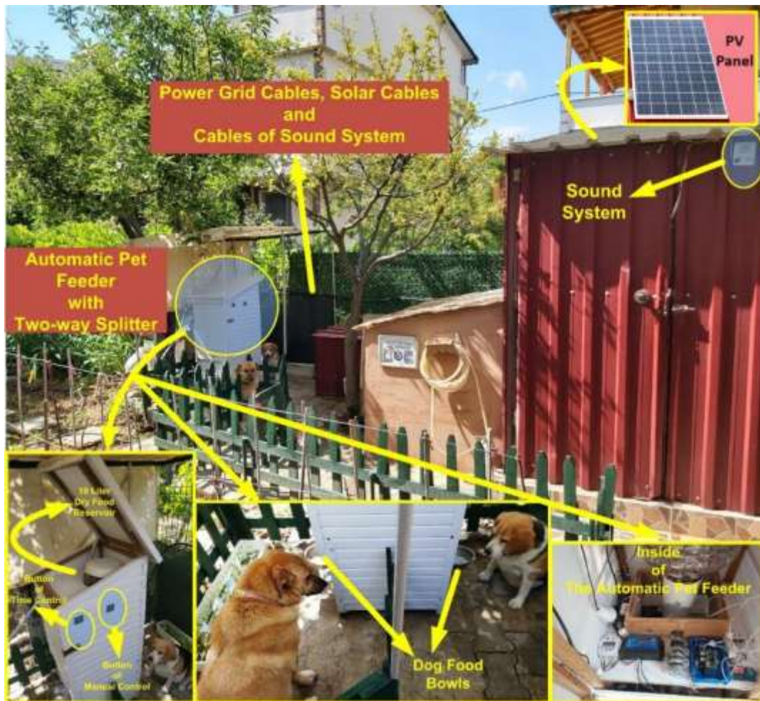
Figure 5. Photograph of the proposed automatic pet feeder
