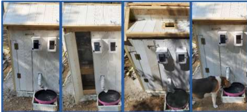
Figure 6. Photographs of the proposed automatic pet feeder
