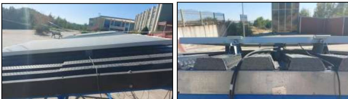
Figure 10. Temperature sensors installed on the PV/T system
