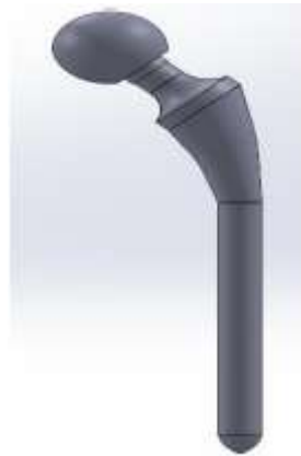
Figure 1. Hip Implant CAD Model
