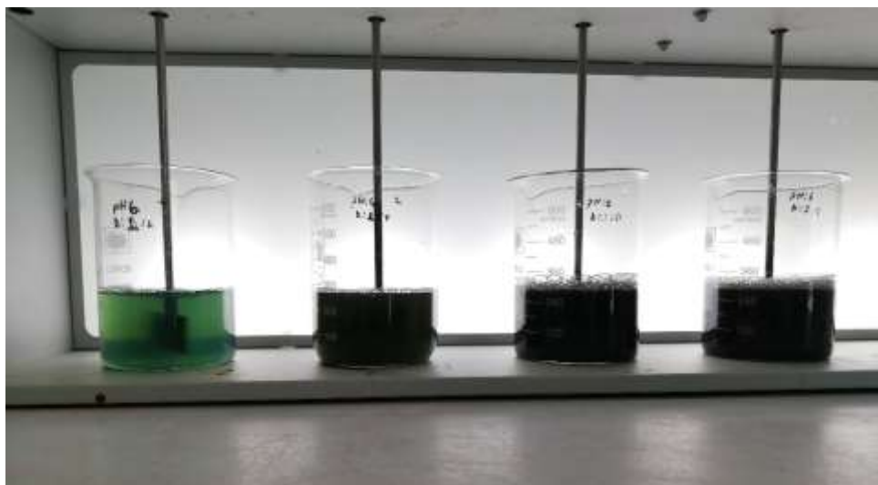
Figure 3. Jar test set-up
